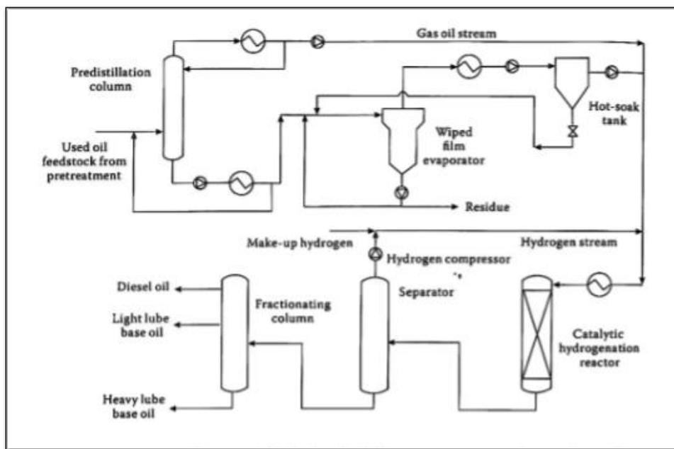
Fig (11) - The KTI Process - Source 1
