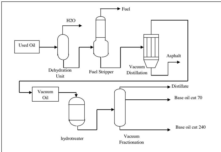
Figure 8 Safety Kleen simplified process flow diagram
