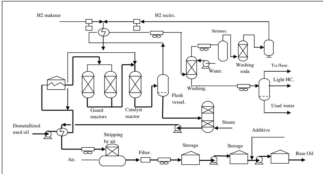
Figure 15 PROP process process flow sheet
