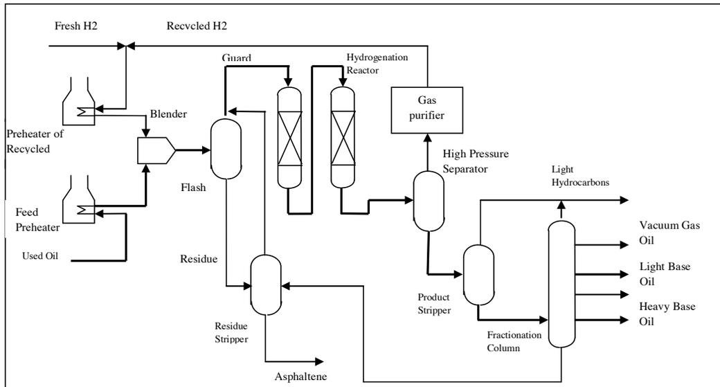
Figure 11 UOP Hylube simplified process flow diagram
