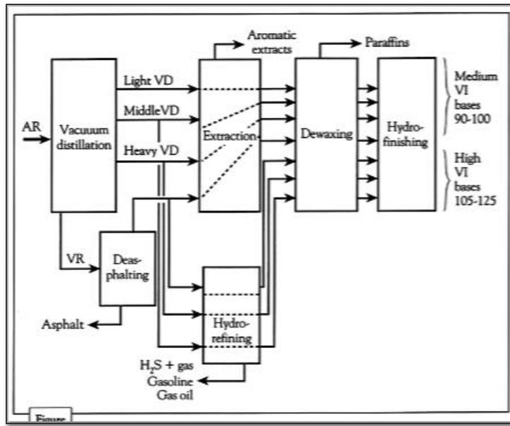
Fig (1) Virgin Lube Processing - Source: 2
