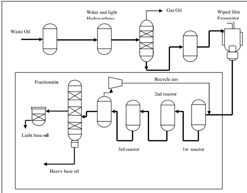
Figure 10 CEP simplified process flow diagram
