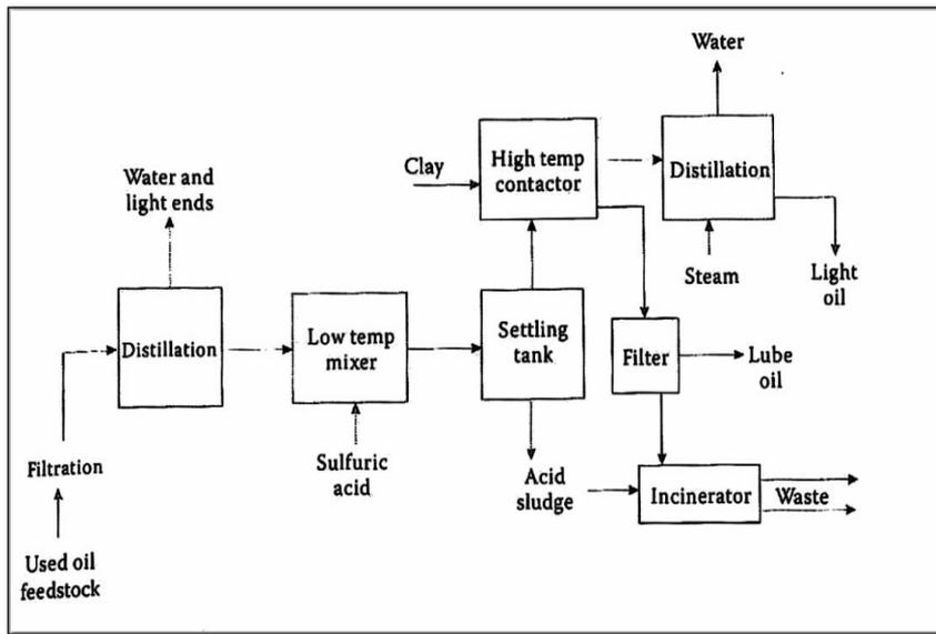
Fig (3) - Acid/Clay Process - Source: 1
