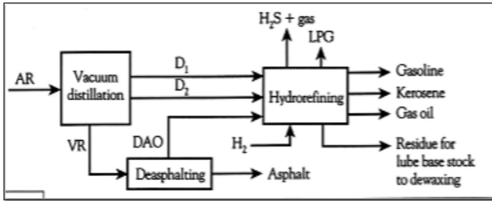
Fig (2) Alternative Virgin Base Oil Processing Source: 2
