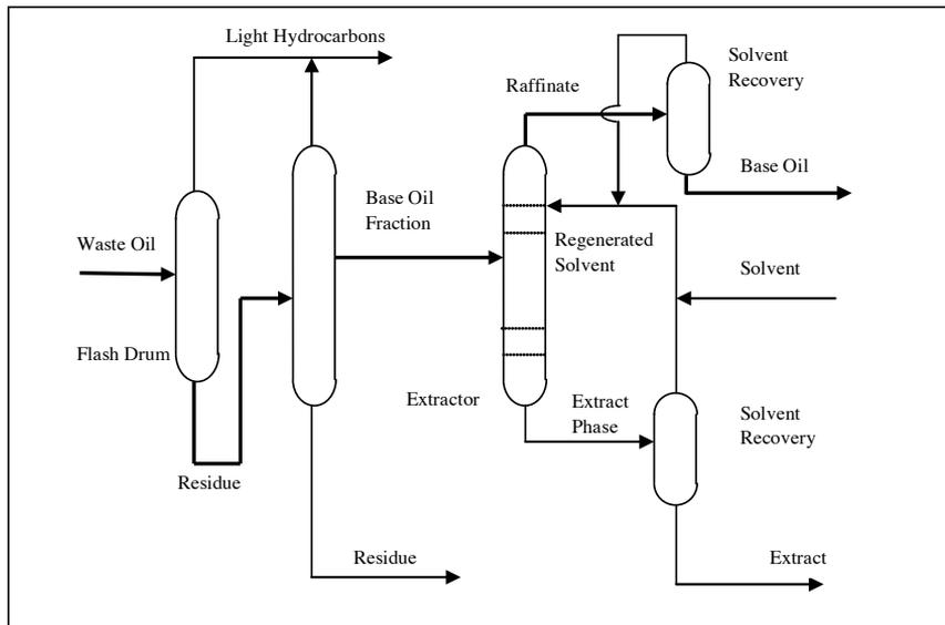
Figure 14 Probex simplified process flow diagram
